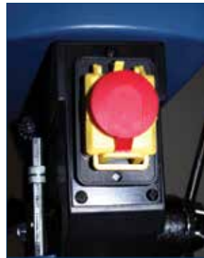
SAFETY LINE INTERRUPT switch requires manual reset in case of power loss.
