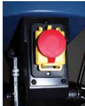
SAFETY LINE INTERRUPT switch requires manual reset in case of power loss.
