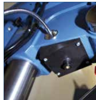
BUILT-IN LASER PROVIDES precise repeat drilling at any angle.
