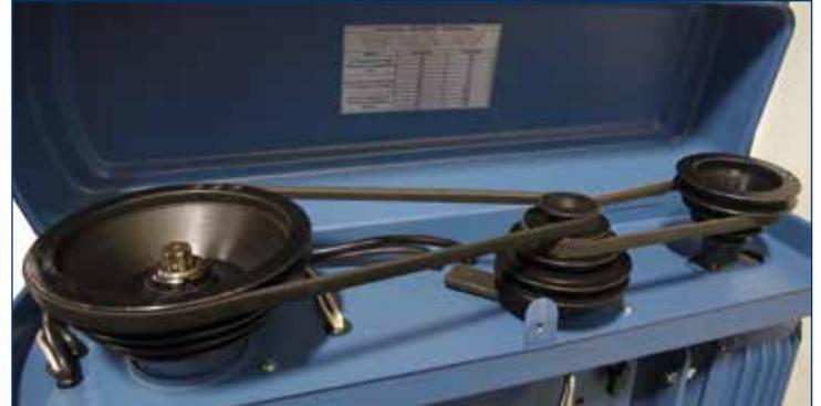
**CAST IRON PULLEYS** reduce vibration. Speed changes are quick and easy.
