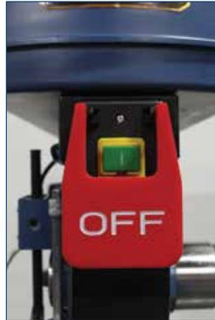
**SAFETY LINE INTERRUPT** switch requires manual reset in case of power loss.
