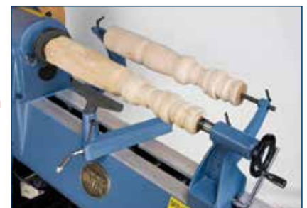
A COMPARATOR JIG included with the lathe, makes for easy duplication.
