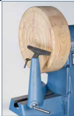
THE OPTIONAL OUTBOARD SUPPORT and tool rest allow a huge 35" swing.
