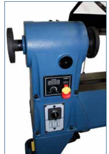
A FREQUENCY INVERTER DRIVE gives a wide range of RPMs from 50 to 3200.
