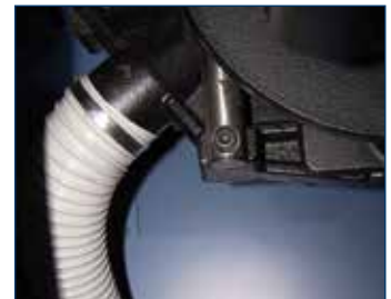
A BLADE ENCOMPASSING DUST shroud joined with the standard 4" outlet.
