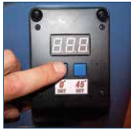
A DIGITAL ANGLE METER takes the guess work out of mitre cuts.
