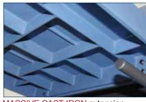
MASSIVE CAST IRON extension wings to support heavy stock.
