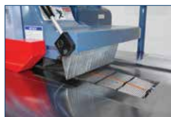
TWO SETS OF anti-kickback fingers ensure operator protection and safety.
