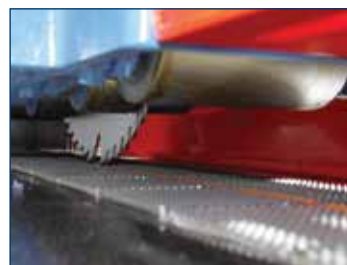
SEVEN PRESSURE ROLLERS hold material securely to the conveyor chain.
