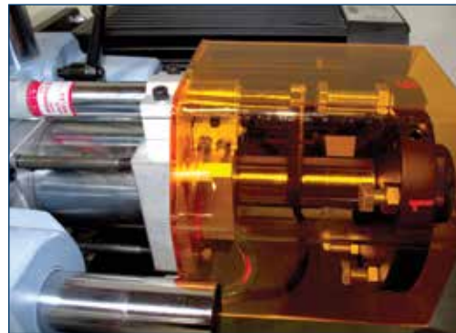
ACCURATE ADJUSTMENT OF BORING UNIT and speed stabilizer provides smooth feeding against the workpiece.
