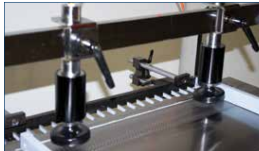
THE BORING UNIT CAN be adjusted from horizontal to vertical drilling by pneumatic setting.
