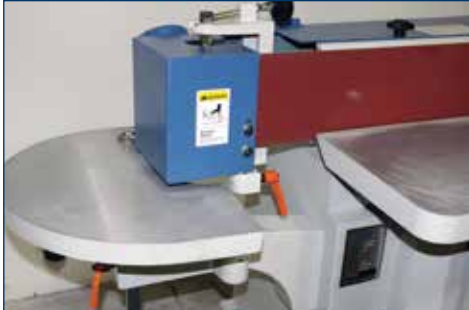
CONVENIENT FULLY ADJUSTABLE end table for contour sanding. Graphite is on platen.
