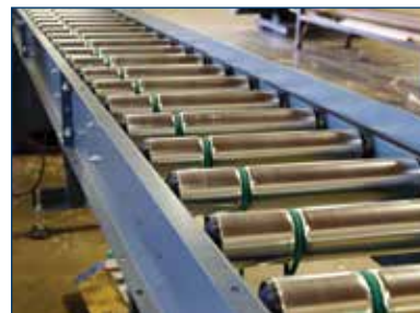
A POWERED infeed roller system aids the operator in feeding timber into the machine. The steel rollers are skewed to keep the material up against the fence prior to entering the machine.
