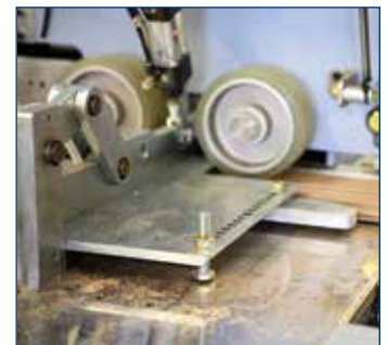
A SOLID PLATE steel clamping system presses the timber flat to the table and hard up against the fence while counter rotating cutterhead machine the tongue and groove.
